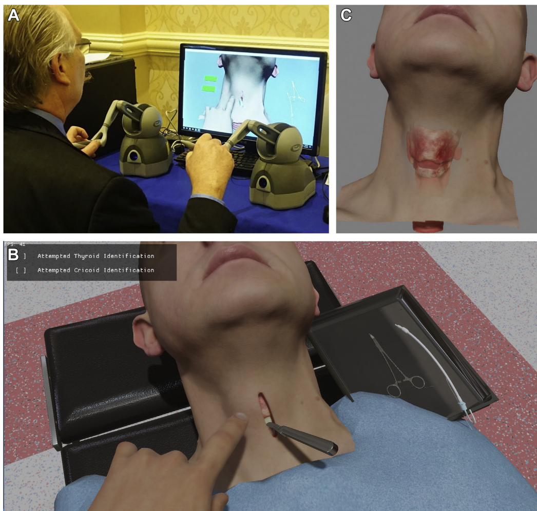
Fig. 1 – VAST-CCT simulator: (A) Haptic-enabled VR CCT simulator, (B) the virtual patient and surgical instruments, and (C) the virtual cricothyroid anatomy are derived from high-resolution CT data and simulated with realistic material properties. (Color version of figure is available online.)
